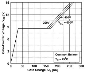
Figure 12. Turn-on Characteristics vs.
