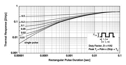
Figure 26.Transient Thermal Impedance of Diode
