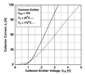
Figure 5. Saturation Voltage vs. Case
