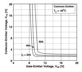
Figure 7. Saturation Voltage vs. V<sub>GE</sub>
