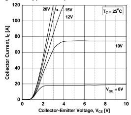
Figure 3. Typical Saturation Voltage Characteristics
