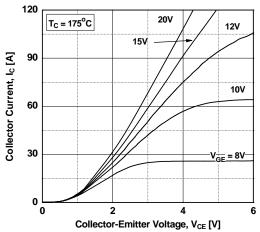
Figure 4. Transfer Characteristics
