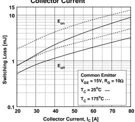
Figure 14. Turn-on Characteristics vs.
